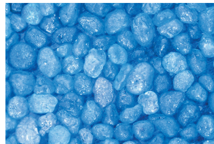
Fig. 5. AquaBond resin-coated proppant reduces formation water, compared to traditional proppants, according to the company.
