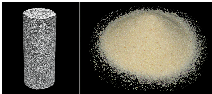
Fig. 7. kRT 100 resin-coated proppant increases microfracture stimulation by forming a bonded proppant pack.
